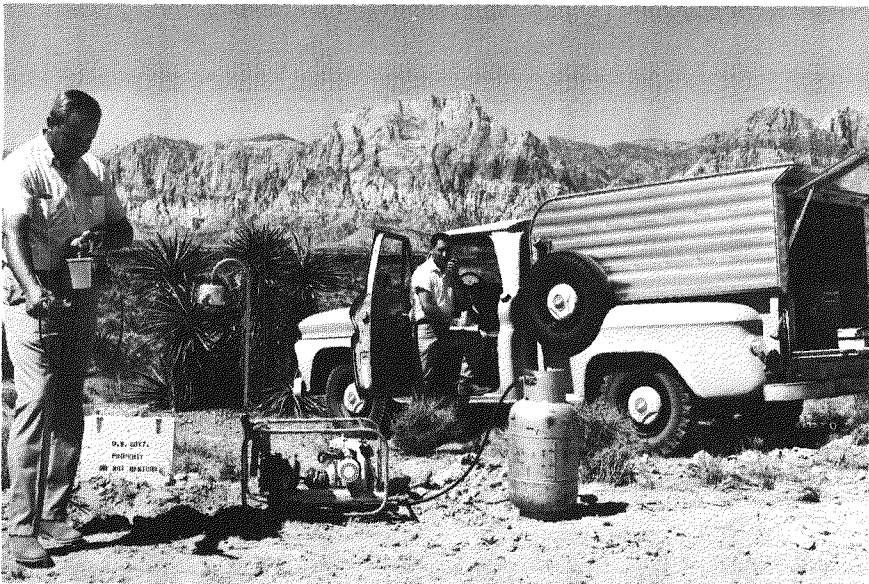
Fig. 8.4 Mobile monitoring station in a desert valley in Nevada. (Bottled gas is used to drive the motor for an air sampler.)
